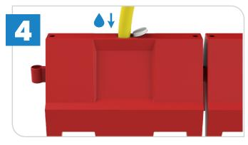
Once you are happy with your interlinking barrier line, it's time to put the water in. To do this, simply open the cap on top of the barrier and use a hose to fill with water. This will help to weigh the barrier down and keep it in place.
