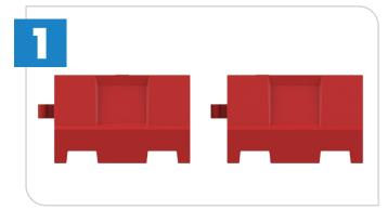
Place the barriers along the perimeter line you want to create. Make sure that they face the same direction. Ensure the ground is stable and the barriers are firmly positioned.
