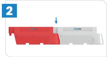
When the 1st barrier is in place, lift the end of the second and barrier lower it into the prong/socket.
