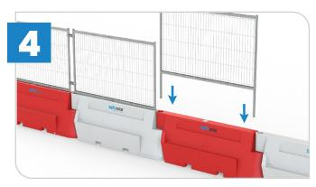
If adding fencing - slot the mesh fence or hoarding panels into the holes at either end of each of the barriers.
