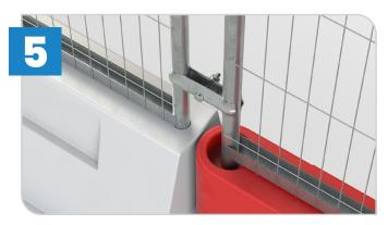
To secure the panels in place, position a coupler between the mesh fence panels and tighten.
