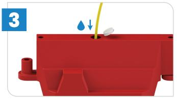
Once you are happy with how the barriers have been linked and arranged, open the white cap on the top of the barrier fill with water (approx. 50 litres).
