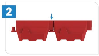
When 1st barrier is in place, lift the end of the second barrier lower it into the prong/socket.
